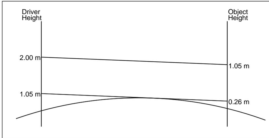
Figure 2/2 : Sightline Requirement in the Vertical Plane
