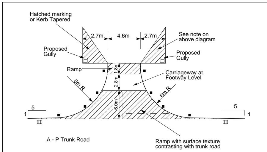
Note: On both of these layouts, where the use exceeds 50 vehicles per hour in the peak, or there is occasional use by LGVs tapers may be considered to be added on both sides of the access on the trunk road. The tapers should be 1:5 and should start and finish 15m from the centre line of the direct access. Where site conditions are difficult, entry radii may be reduced to 4m as a Relaxation.
