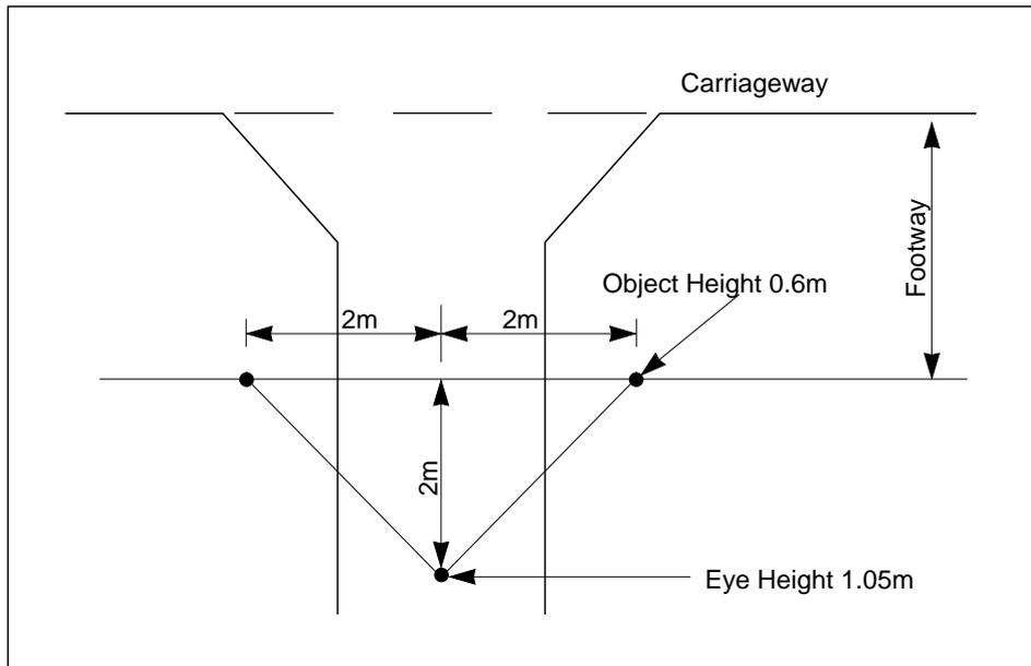
Figure 2/2 : Visibility at Back of Footway Crossing
