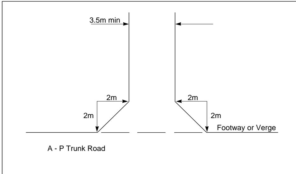
Where field accesses are frequently used by wheeled vehicles, consideration should be given to constructing a hardened approach strip to assist in the removal of mud from tyres and equipment prior to entering the trunk road.
